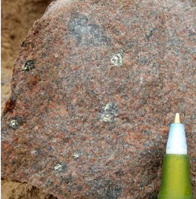
Figure 9-9: Strongly K-altered Berkey Phase with coarse chalcopyrite grains
